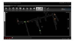
MineTracker software provides realtime and last known location reporting using imported mine maps. Collision avoidance can be included in vehicles. MineTracker has the ability to monitor speed, telemetry, oil pressure, temperature and more.
